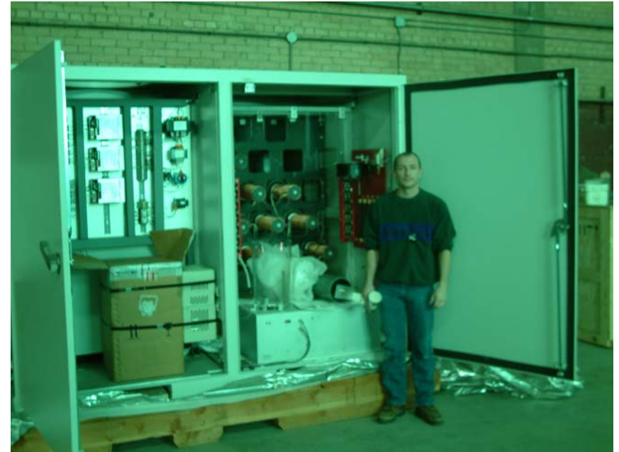
MALE Modulator Chassis, 6'x9' footprint. Electrical requirements; 480V, 250A, 3 phase.
